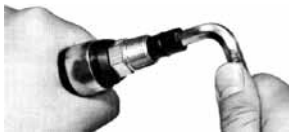
2. Position hose end on SHELL (A) flush with groove (see arrows).
