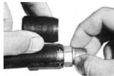
3. Insert FITTING (B) into groove and position SHELL (C) opposite SHELL (A).
