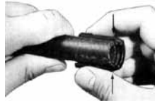
2. Position hose end on SHELL (A) flush with groove (see arrows).
