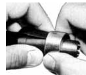
4. With assembly in hand, squeeze forward ends of shell and push and twist RETAINING RING (D) over shells to its final position as shown by arrows.
